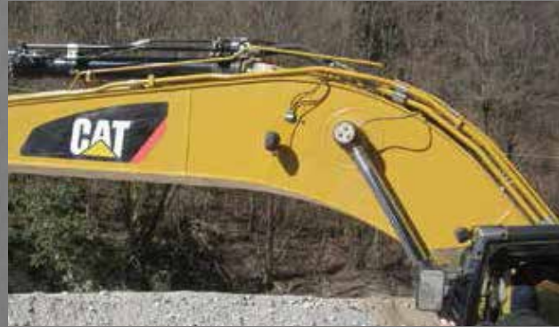
ANGLE SENSOR ON EXCAVATOR
